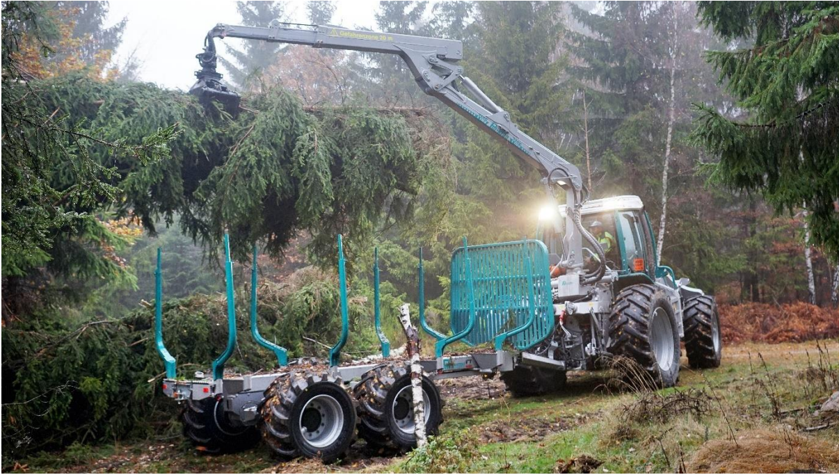
Image 5: Pfanzelt Professional P17 forwarding trailer with 4-wheel hub drive
