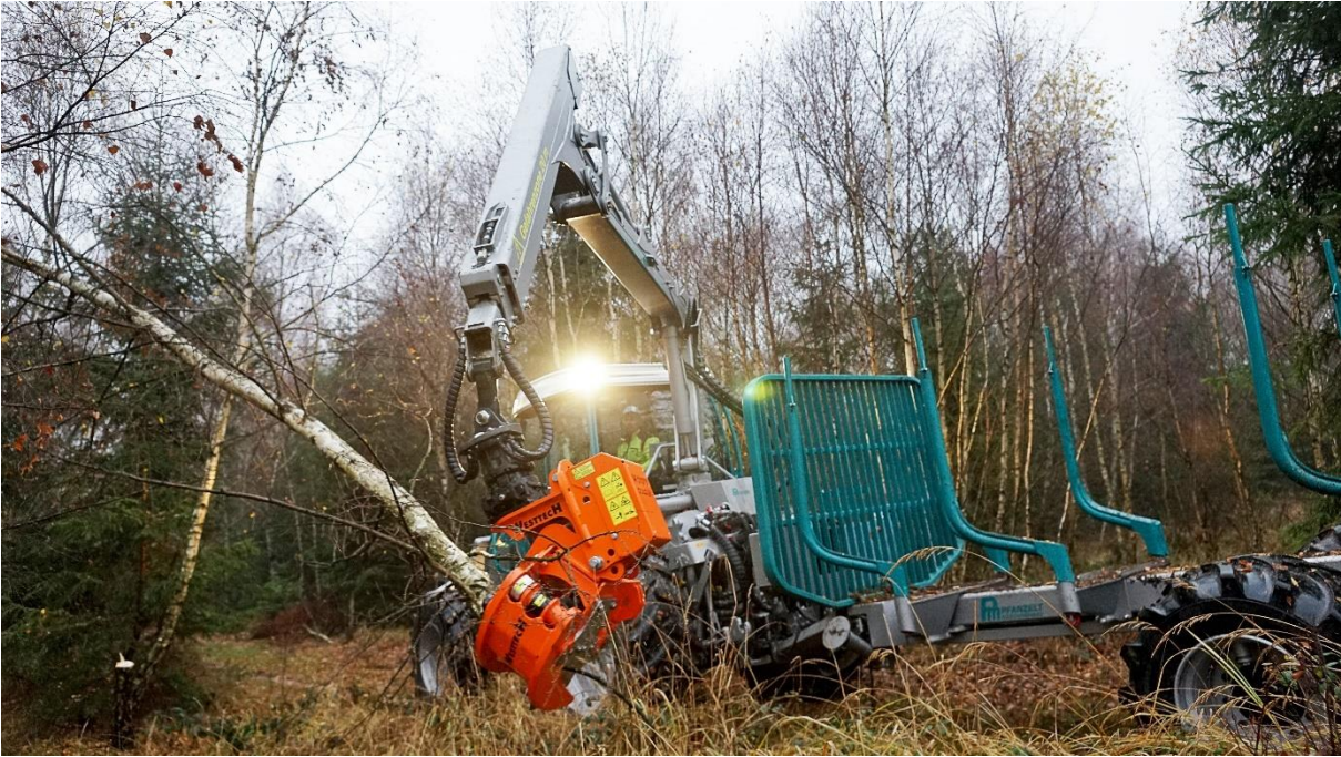
Image 3: In addition to the timber grippers it is also possible to install attachments, such as the Westtech Woodcracker
