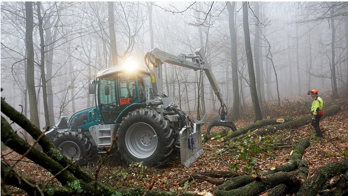
Image 2: Cable winch and forestry crane have been installed at a favourable centre of gravity over the rear axle
