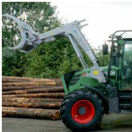
Front stacking shield unit
