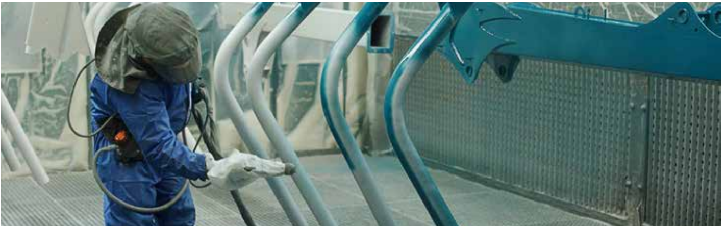
After sandblasting, we paint the parts in house.
