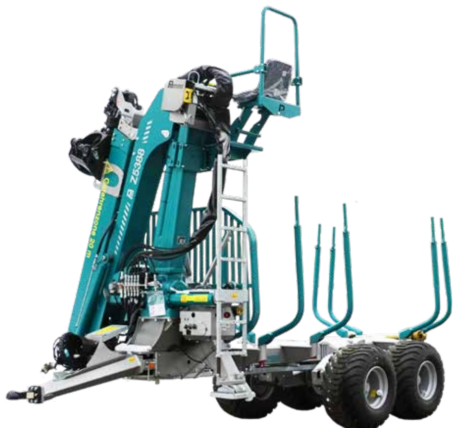
Pflanzelt Profi forwarding trailer P13 with Z-crane 5388, high seat and radio control
