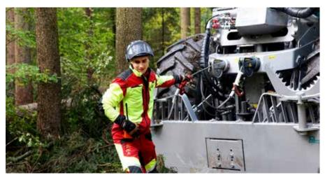
On the Pm Trac, Pfanzelt's winch units are mounted under the forest crane above the rear axle.
